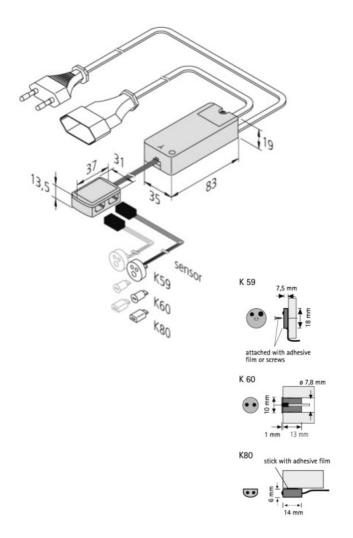
Description: contactless door switch for connection of class II equipment for luminaires, mains cable 3m with Euro plug, switching line 0,3m with Euro coupling, two sensor cables 3m with sensor K60, switch function: opening one of the two doors switches the light on and closing the doors switches it off again.
