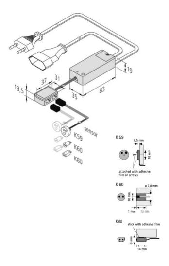
Description: contactless door switch for connection of class II equipment for luminaires, mains cable 3m with Euro plug, switching line 0,3m with Euro coupling, two sensor cables 3m with sensor K60, switch function: opening one of the two doors switches the light on and closing the doors switches it off again.
